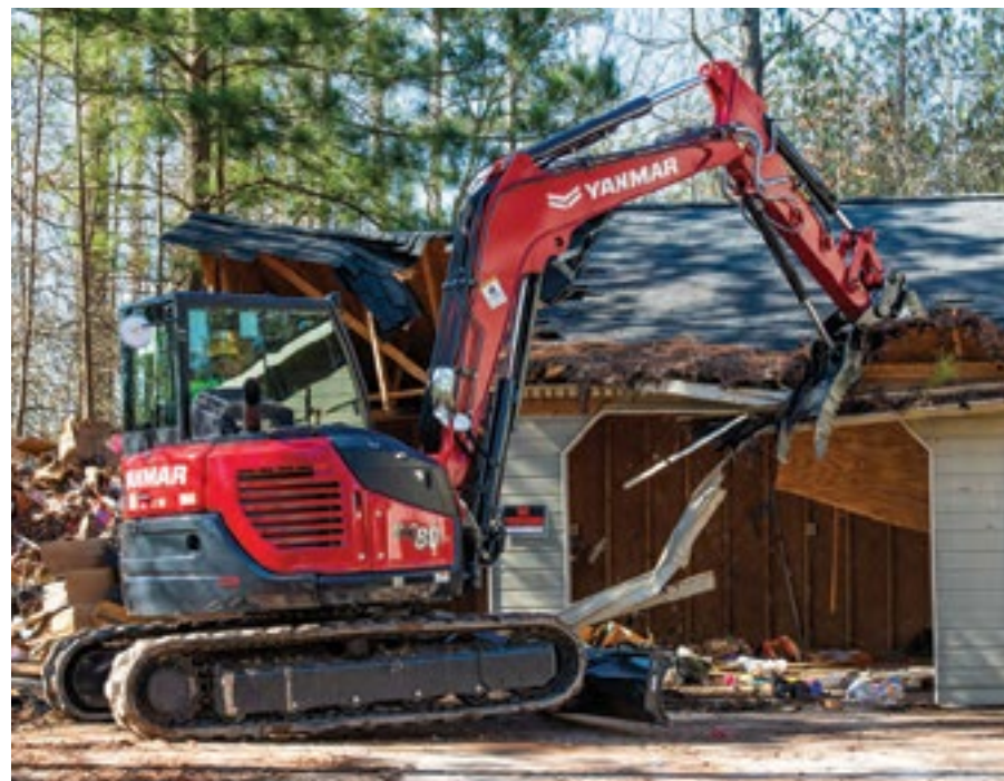
Cabs are seeing improvements in ergonomics, such as switches and displays that are more viewable and controls that are easier to use. Enhanced attachment coupling options also improve efficiency on the job site, with hydraulic options allowing switching attachments without leaving the cab.
