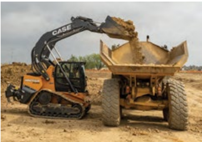
In its loader configuration, the Case Minotaur DL550 features a 5,500-pound rated operating capacity (50 percent of tipping load) with 12,907 pounds of breakout force. It features a vertical lift that operates in the ISO control pattern.
