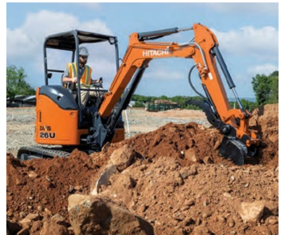
Many Hitachi compact excavator models feature power/economy modes that are usually only available on larger excavator models. These modes allow the operator to match the engine speed to the job.
