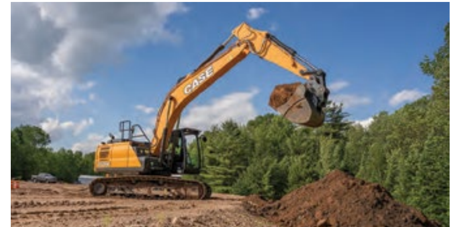
The new Case E series excavators feature working modes that incorporate throttle selection for greater control of machine performance in varying job site conditions. In the past, engine throttle speeds were not adjustable within these working modes.
