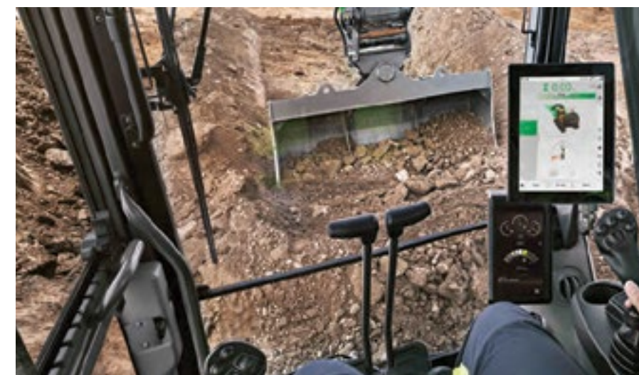
Assistive software, like Volvo's Dig Assist, makes work faster and easier by allowing the operator to automate some of the most common tasks such as leveling and sloping, creating layers of different materials or weighing the material moved.
