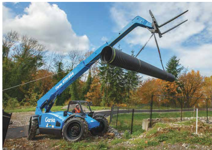
Telehandler fork attachments outfitted with hooks or clevises allow users to lift awkward loads safely and efficiently.
