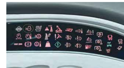
Dashboards and instrument clusters have icons that light up when there are issues. Here, the second icon in the top row warns that coolant needs to be topped off.
