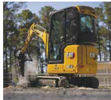
The Cat 301.9 mini excavator (left) and the Cat 906 compact wheel loader are expected to be the first commercially available battery electric equipment models from Caterpillar. The units will feature scalable battery systems that can be adapted for other types of equipment and uses and will have onboard charging systems.
