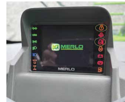
Instrument clusters on heavy equipment, just as on automobiles, have many icons that light up when there are engine issues. For example, when these two icons are lit at the same time, stop operation. Turn off the vehicle. There is a major issue with the cooling system.
