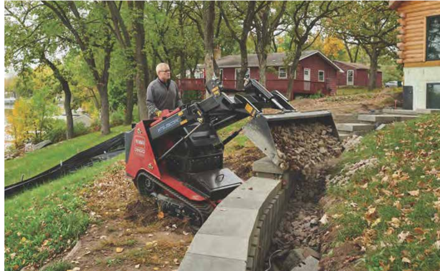
The most enticing characteristic of compact utility loaders is their versatility. Depending on the manufacturers, users can turn them into virtually any machine by switching out the attachment with one of many others.
