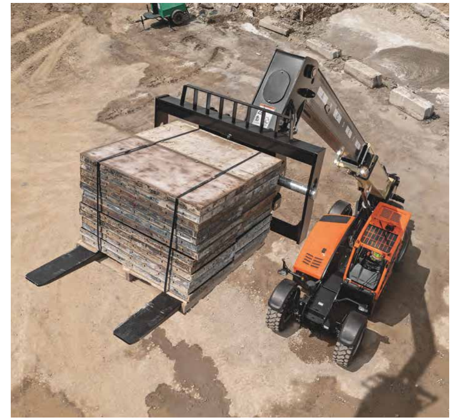
Telehandlers are called tool carriers for a reason; they can handle a wide range of hoisting and material-handling applications because of the large variety of attachments with which they can be equipped, from buckets, carriages and truss booms/lift hooks to specialty attachments like tire handlers.
